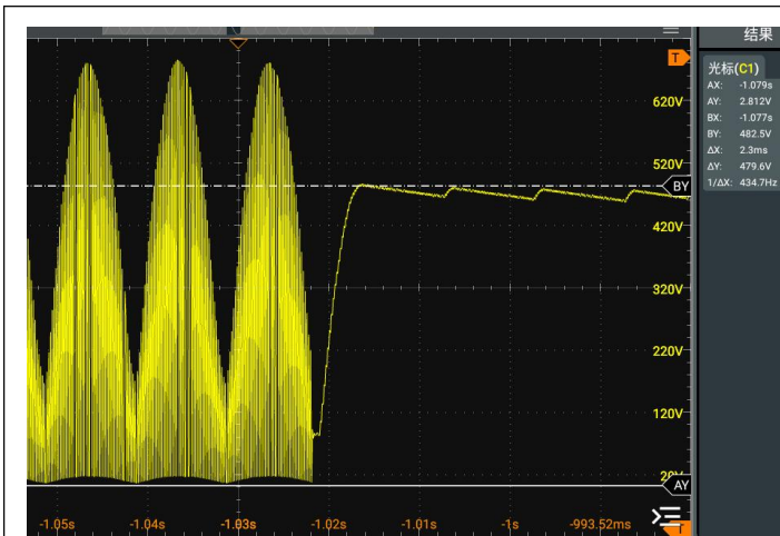
Trigger the OVP : V_{in}=331Vac, DC=24V 2.5A
