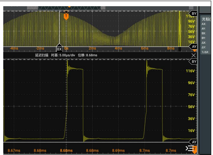
2#: V_{in}=300Vac, DC=24V 2.5A, V_D \approx 138.1V
