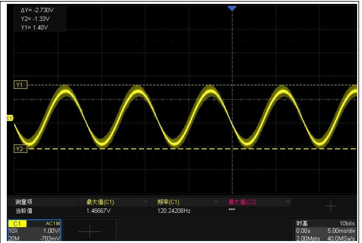
Typical Ripple Voltage of V_{OUT}=24V , I_{OUT}=1.25A@230V_{ac} FULL load (Power frequency ripple)
